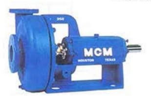
250 Series Pumps feature a 21st shaft, replaceable shaft sleeve and stuffing box and a thicker concentric housing. This series is available in eight sizes (2x3x13, 3x4x13, 4x5x14, 5x6x11, 5x6x14, 6x8x11,6x8x14 and 8x10x14).
